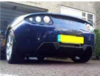
Dash CAE 3D printed a diffuser floor, seen on a Tesla underneath the license plate, on its Fortus 400mc Production System.
