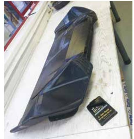
A full-size diffuser floor 3D printed in black ABSplus on the Fortus 400mc Production System
